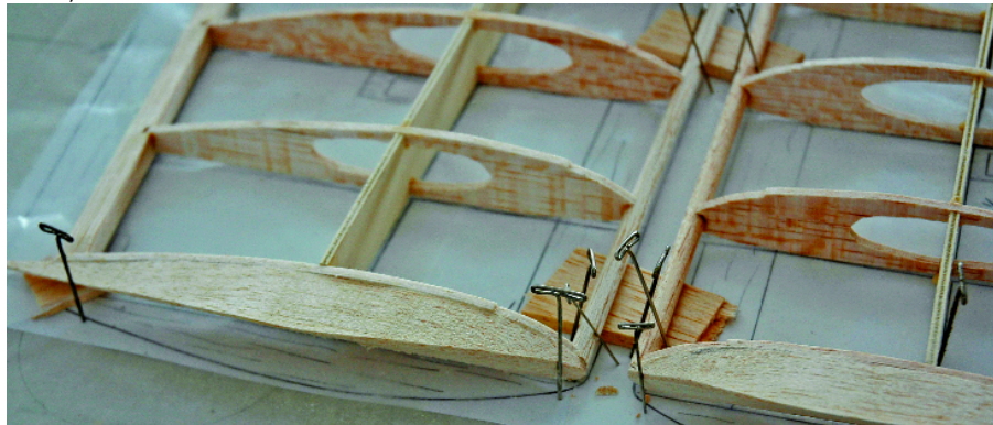
The wing panel halves are built directly over the full-size plans. It's hard to build a warp into this wing!
