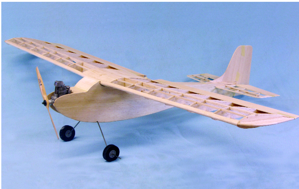
The wing ribs are flat-bottomed, allowing accurate assembly on a flat bench. This is a logical first built-up model.
