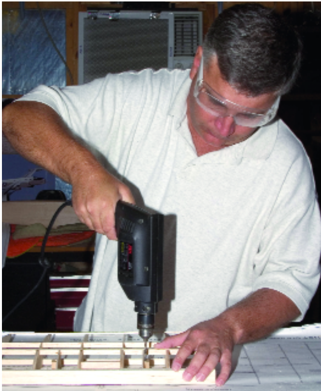
Before sheeting the top of the wing center-section, drill the holes for the landing-gear wires through the landing-gear mounting blocks using the vertical piece of grooved block as a guide.
