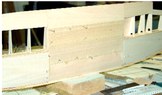
Drill a 1/4-inch hole in a large block of wood and insert the 1/4-inch wing-mounting dowel. This holds the wing in a vertical position, aiding in construction.
