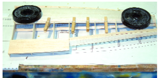
Glue the top sheeting to the LE only first. After the glue dries, wet the top sheeting with water and ammonia to make it more flexible.
