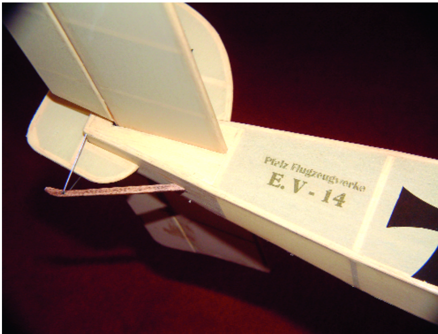
In this view of the tail area you can see the tail-skid detail and some of the graphics that lend to the model's scale appearance.
