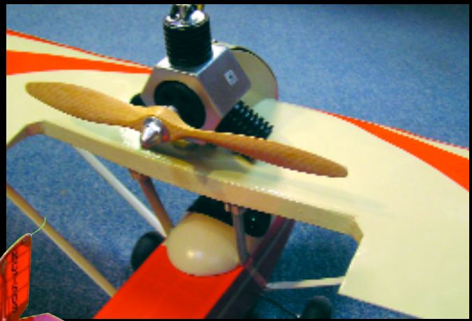
The dummy three-cylinder engine covers the functional Nippy Black electric motor.
