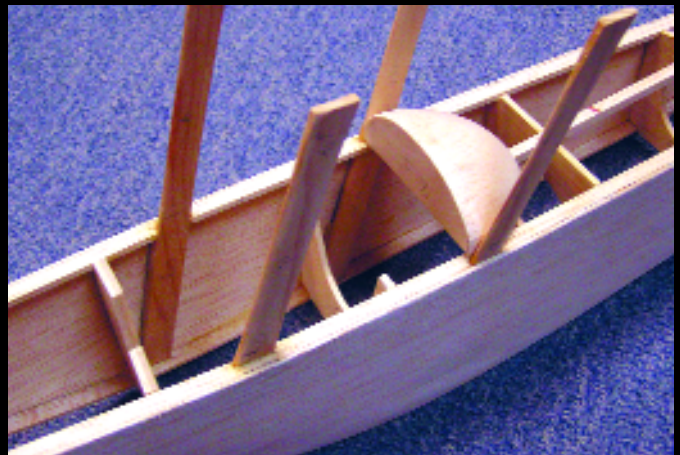
The four cabane struts glue to the fuselage sides and are plenty rigid and strong.
