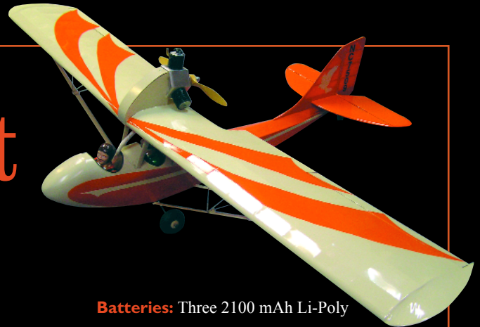
The four cabane struts glue to the fuselage sides and are plenty rigid and strong.
