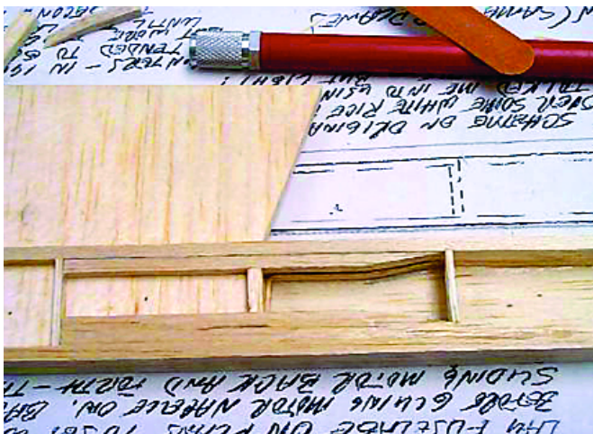
The 1/8 square doublers at the rear of the pylon, extending fore and aft, will provide needed strength in this high-stress area. DTed landings are sometimes rough and tumble and require judiciously beefing up the structure in key locations. Smith photo.
