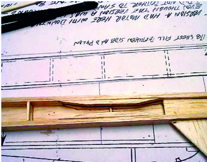
The fuselage is minimal in terms of weight and cross-section and can be strengthened by adding 1/8 square doublers under the stabilizer mount area before adding the left-side fuselage sheeting. Smith photo.
