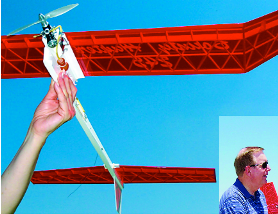
Left: The new 245-square-inch Bounty Hunter retains the original's classic lines and construction features. This prototype rendition by Larry Kruse uses a canted engine mount to preserve the fuselage profile. Kruse photo.
