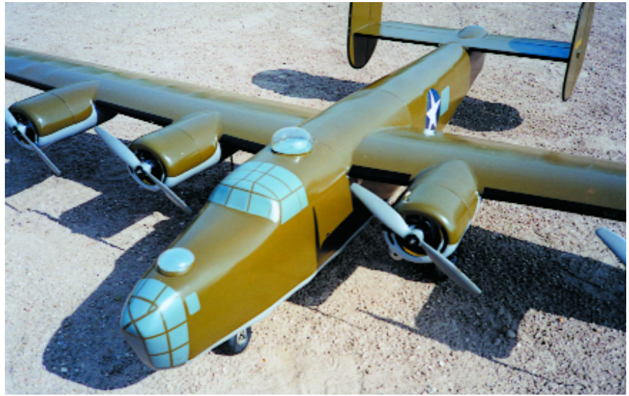
Painted-on window and blister detailing makes building and finishing this model much easier!
