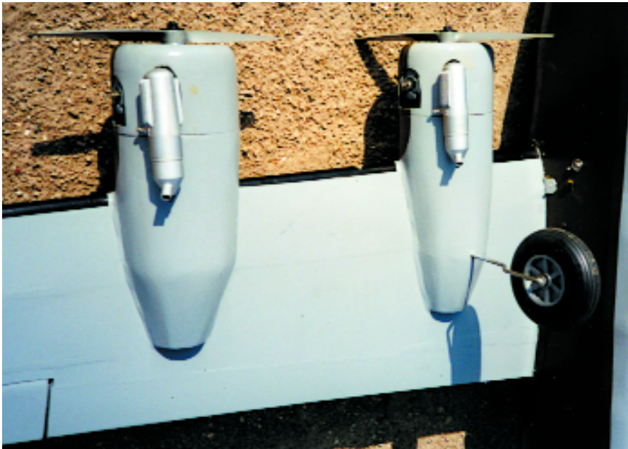
The four O.S. .10 FP engines fit snugly into their respective cowls, and the mufflers are nestled neatly against the bottom of the nacelles.
