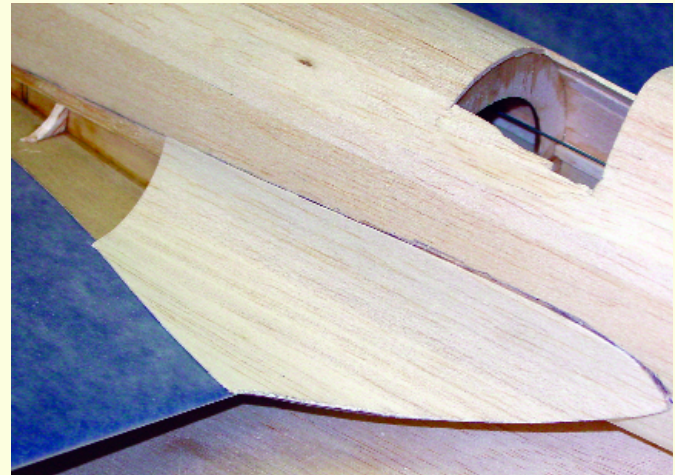
The top of the wing fairing is planked with balsa. Take your time here and achieve a good fit.
