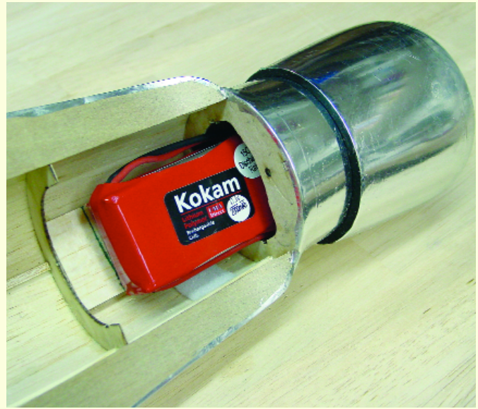
The battery pack will probably need to be positioned somewhat forward, as shown. Provide a secure hold-down.
