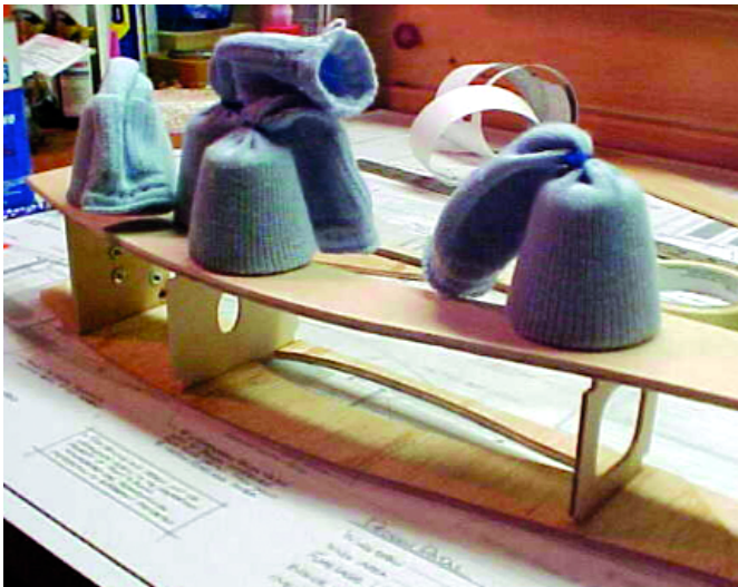
Weights are used to hold the fuselage sides and forward formers in position while the glue dries.
