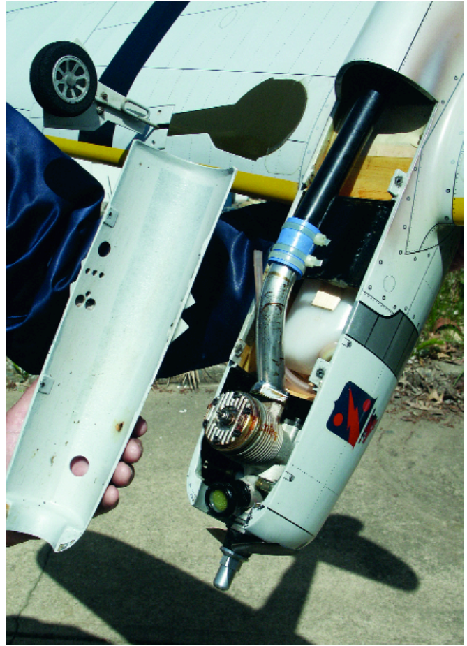
The P-47's engine bay. A PA .61 fitted with a Smith and Wernage carbon-fiber tuned pipe supplies power. Notice plastic uniflow clunk tank. There's lots of room in this model.
