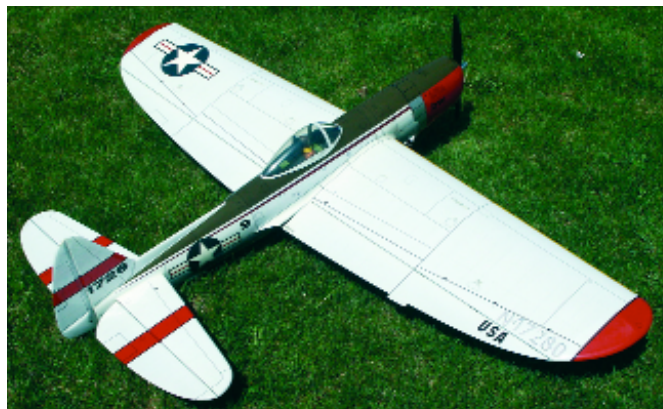
This bubble-canopy version was built at the same time as the featured razorback version. It has a blunter LE and forward TE sweep.
