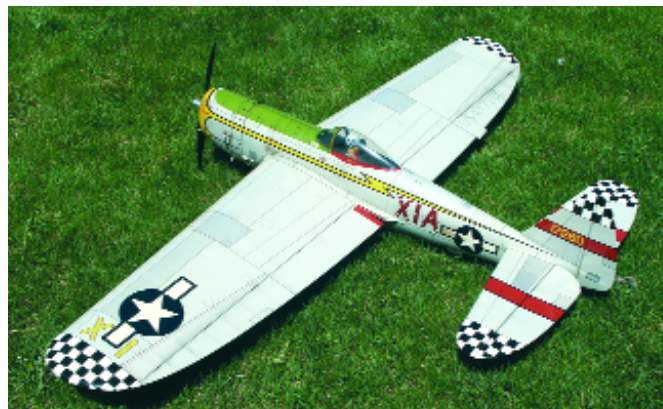
Another bubble-canopy version, with a slightly longer tail-moment arm, slightly shorter nose-moment arm, and slightly wider fuselage.
