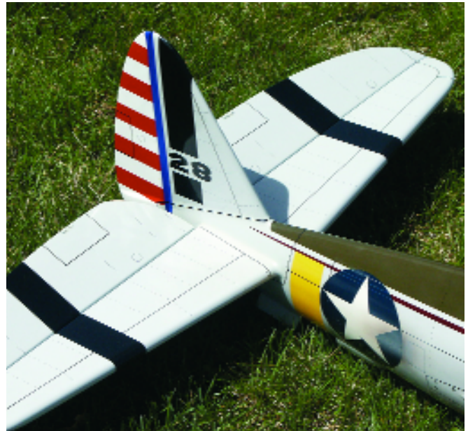
The stabilizer and elevator are made from sheeted balsa cores with support ribs. Text has details on this procedure.
