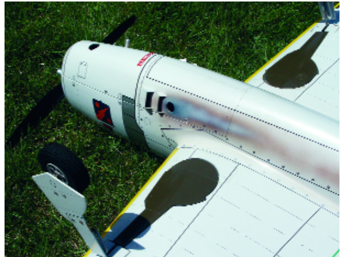
Bill used an airbrush to spray the simulated exhaust stains on the sides of the lower fuselage. It gives a great scale effect.
