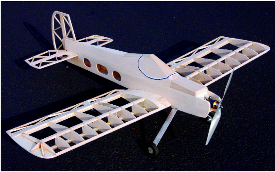
Looking at the bare framework you can see that there is no wing LE sheeting, but partial ribs are used on the LE sections. Ailerons and all tail surfaces are built up.
