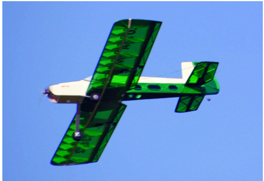
Transparent MonoKote finish reveals the lightweight wing, tail, and fuselage structure. It adds up to performance!
