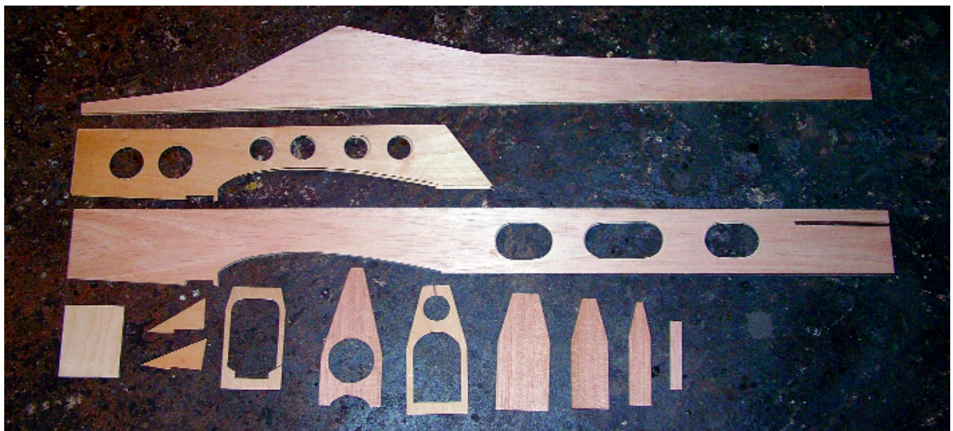
The fuselage parts are cut out and ready for assembly. There are few parts in this simple-to-construct aircraft.
