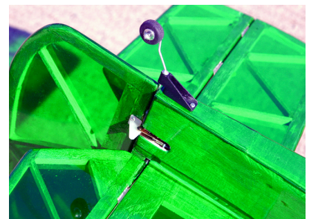
A close-up showing the rudder control horn and the steerable tail wheel.
