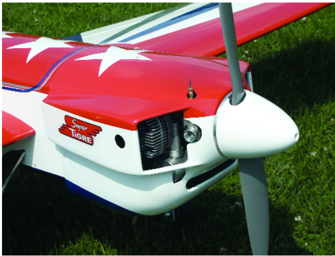
A close-up reveals a neatly cowled-in SuperTigre 2300 engine. A Bison Pitts-type muffer was used.
