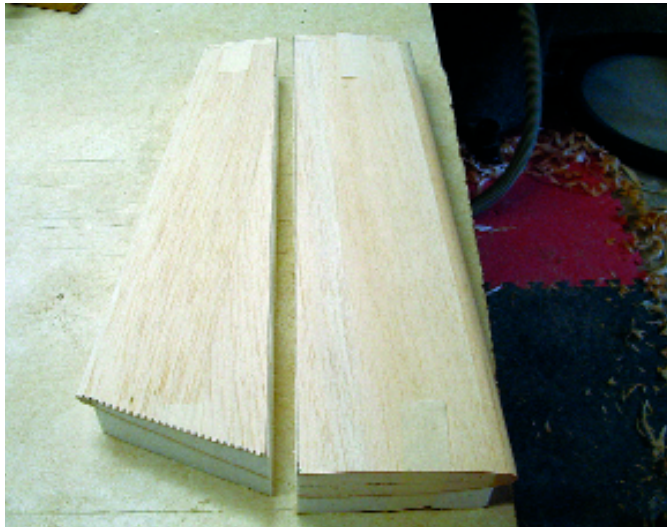
One of the elevator and horizontal stabilizer halves separated and capped at the LE and TE.
