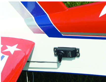
Individual servos on either side of the fuselage aft end actuate the individual elevator halves. Simple and accessible!
