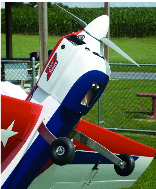
A bottom view of the nose area reveals the curved aluminum landing gear and the exit tubes of the Brisson muffer.
