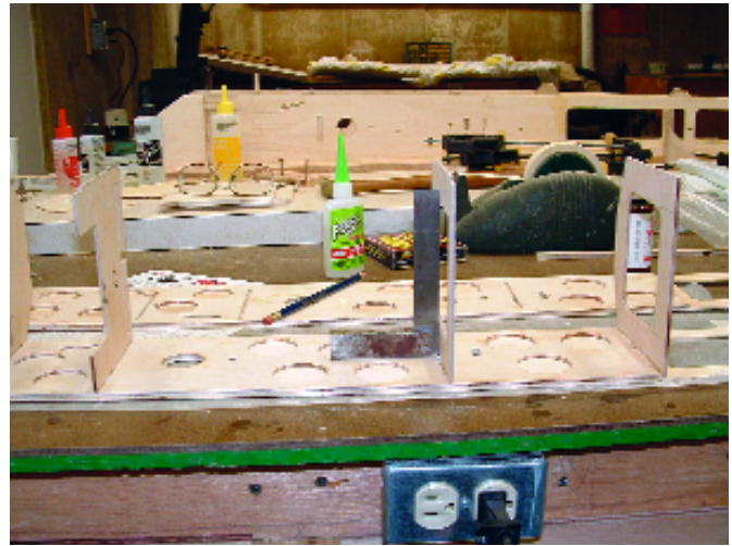
Formers F1, F2, F3, F4, and the landing-gear plate (LGP) are glued in place and set with a square.
