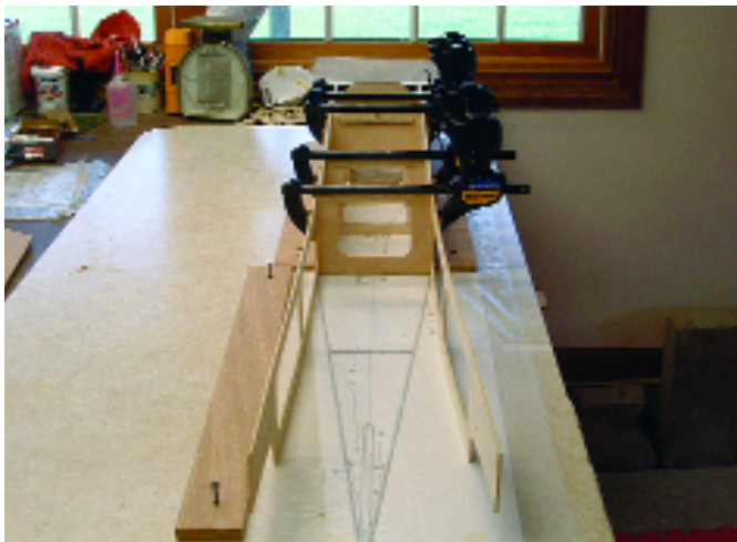
The parallel forward section of the fuselage is joined over the plans with formers FW2, F1, F2, F3, F4, and the LGP in place.
