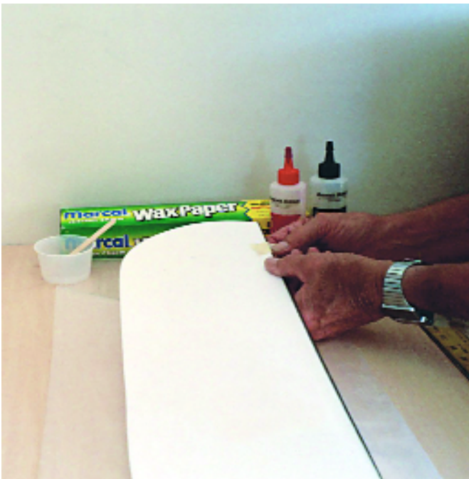
Use epoxy or foam-safe cyanoacrylate to attach 1mm x 3mm carbon-fiber strips to both wings' LE and TE. Hold the carbon fiber in place with masking tape until the glue dries.
