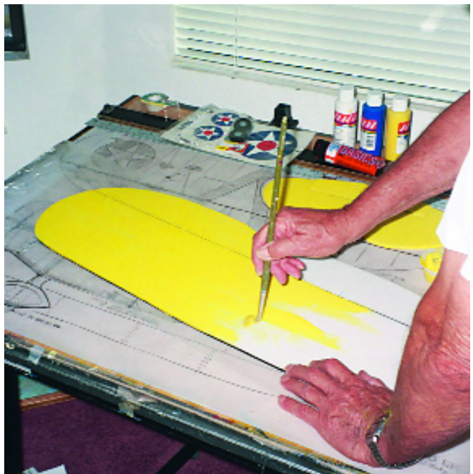
Paint all parts with acrylic paints (available at craft stores) before final assembly. Thin the paint with water and apply with a soft watercolor brush.
