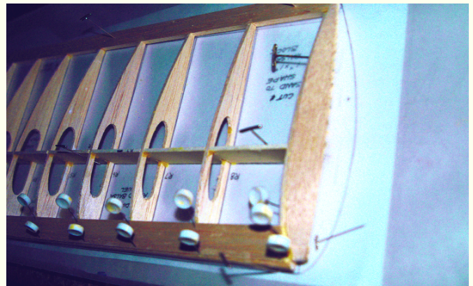
The spar and LE sheeting are shown installed. This makes the wing rigid and resistant to warps.
