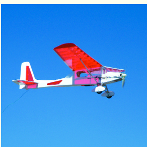
The basic wing is easy to build because the flat-bottom airfoil allows the ribs to sit flat on the plans.
