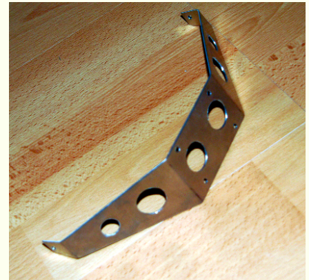
The landing gear is made from flat sheet .040-inch-thick aluminum. The author polished his nicely!
