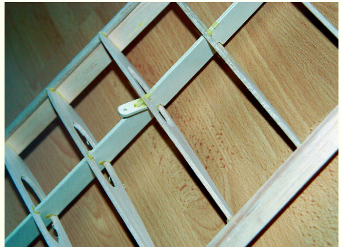
The 1/16 plywood wing-support strut attachments anchor to the bottom of the SkyStroller's wing.
