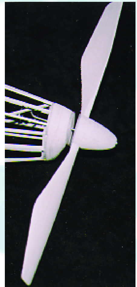
The nose-block assembly has been fitted to the fuselage. You can see the downthrust that is built in.
