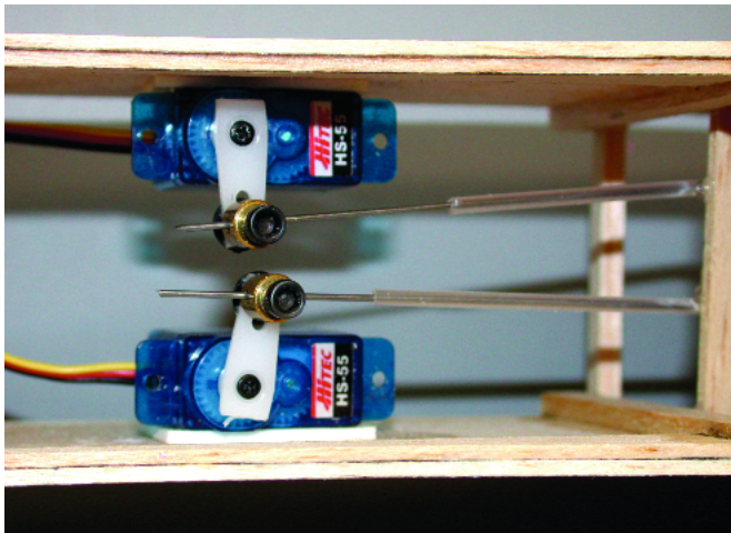
Both Hitec HS-55 servos employ Du-Bro regular-size E/Z Connectors on their output arms, allowing easy adjustment of both control surfaces to their neutral positions.
