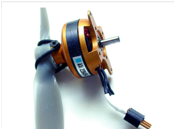
Close-up of AXI 2204/54 Outrunner brushless motor, which runs propeller directly. No gear train is required. Prop-saver mounting uses small rubber O-ring.
