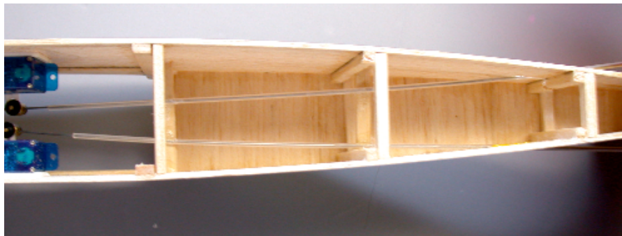
Both control rod nylon sleeves (tubes) were installed between servo and control surface before sheeting bottom of fuselage. Cement sleeves to support pieces to prevent flexing.
