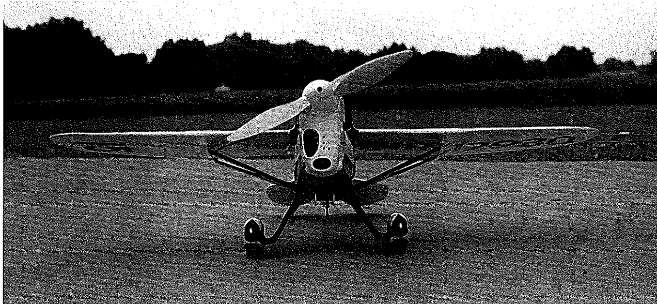
From the front you can study the cowl air-inlet openings. The wheel-pant fairing shape is also visible in this view.
