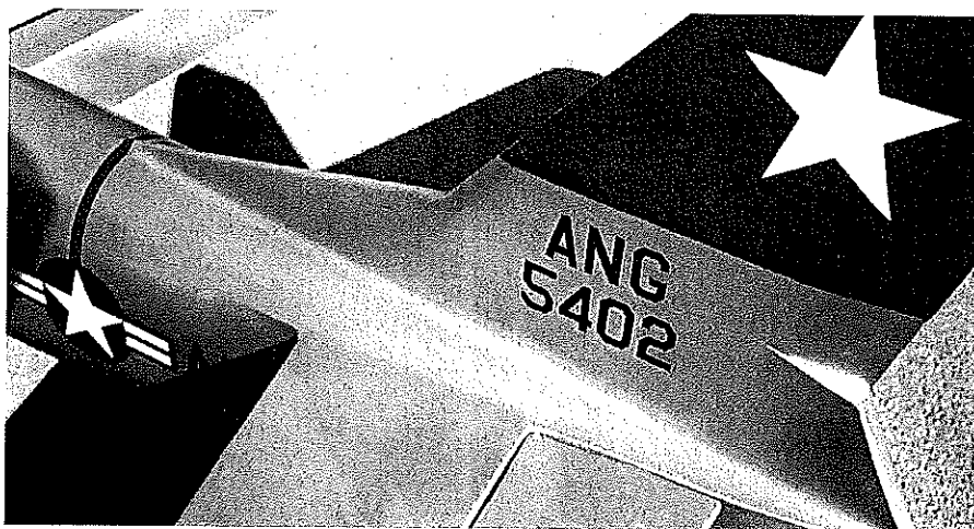
The fuselage's contour changes from convex to concave around the stabilizer. The wide section below the rudder on the full-scale F-86 held a parachute.
