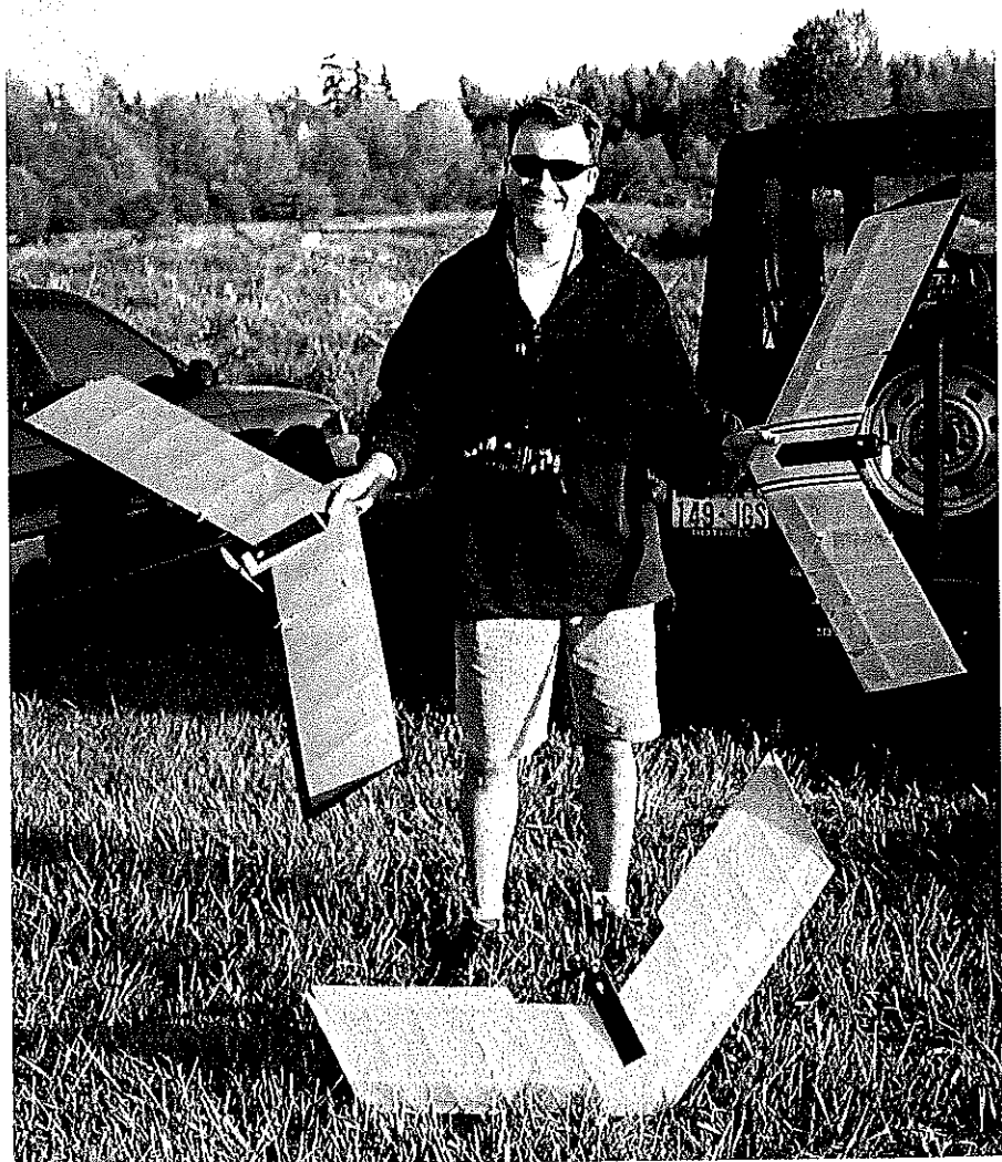
The author displays a collection of his electric-powered wing designs. The model at his feet is a geared 280 version, complete with landing gear.
