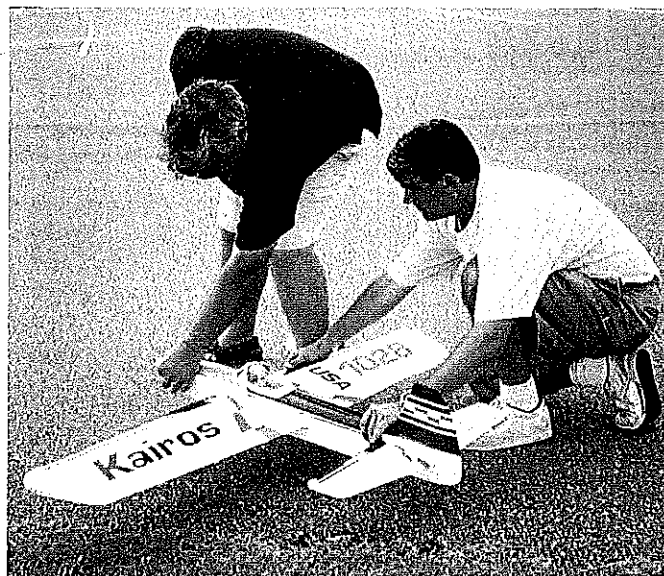
The upright-mounted engine makes starting a breeze. Tom is using a Bolly three-blade 12 x 6 propeller. It's a nice package.
