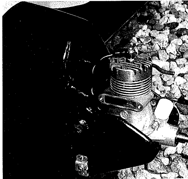
A Stuka Stunt Works tuned O.S. .35 engine is nestled in a rigid mount. Notice the remote glow-plug wire and the plug-in jack system.
