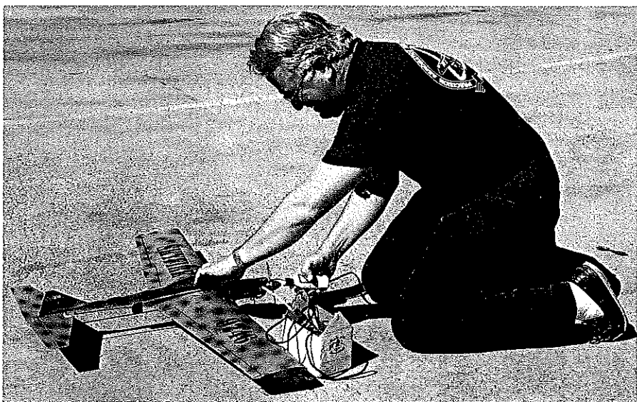
The author uses a Miller RC electric starter to wind the Norvel BigMig .05 engine.
