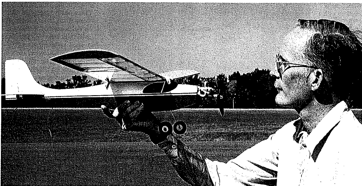
Wing attaches with rubber bands, which "lacks beauty" but is practical for sometimes-rough flying sites.
