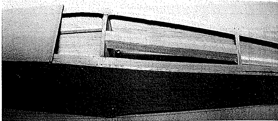
Towhook block laminated from \frac{3}{16} \times \frac{3}{8} spruce and epoxied between F2 and F3.
