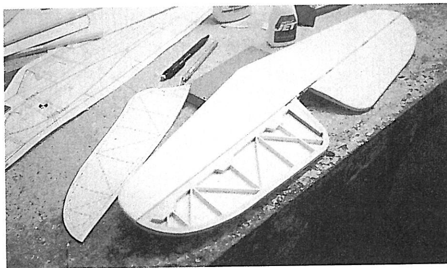
Diagonal ribs are used on elevator to provide extra stiffness as done for flaps.
