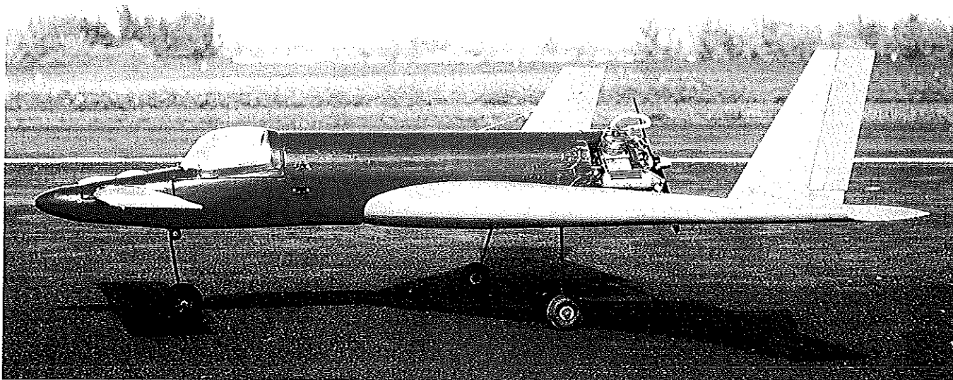
Rear Wind is based on Jim Parrish's full-scale Dart. Model retains Dart airfoil but planform has been modified.
