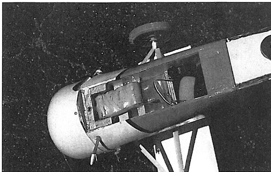
The 1,700-mAh battery pack is well forward. Mustard-jar fuel tank also visible.
