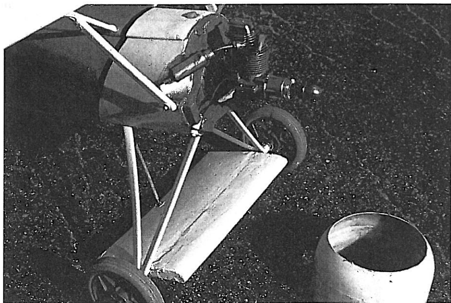
Cowl is cut from a one-gallon mayonnaise jar. Engine is an Enya 46 four-stroke.
