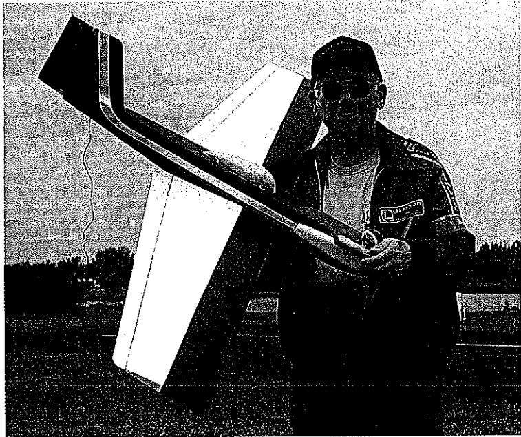
Phil Greenberg and prototype Tradition. Fuselage has been "stretched" a bit in this version. Wing area 710 square inches.
