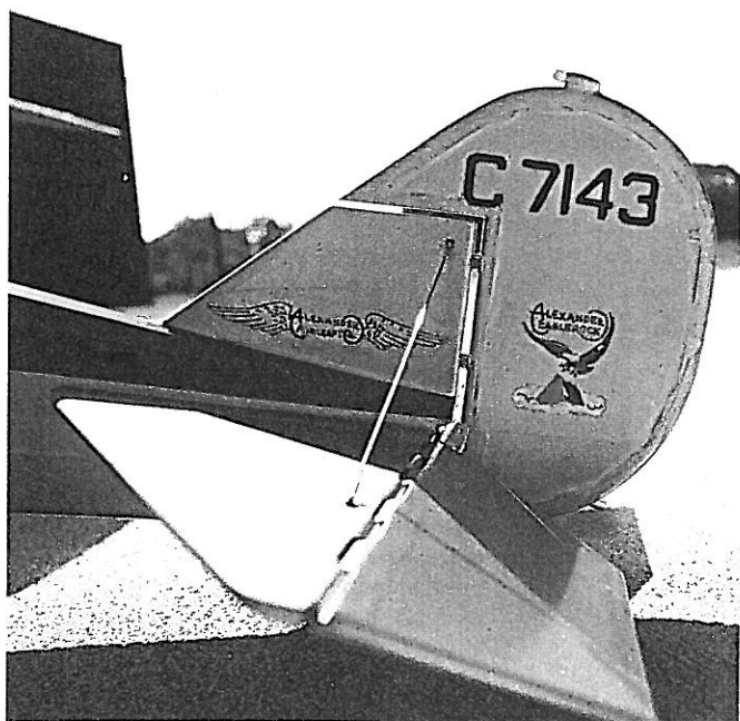
Alexander Aircraft Company logos on fin and rudder. Note tubing and wire elevator hinge system.
