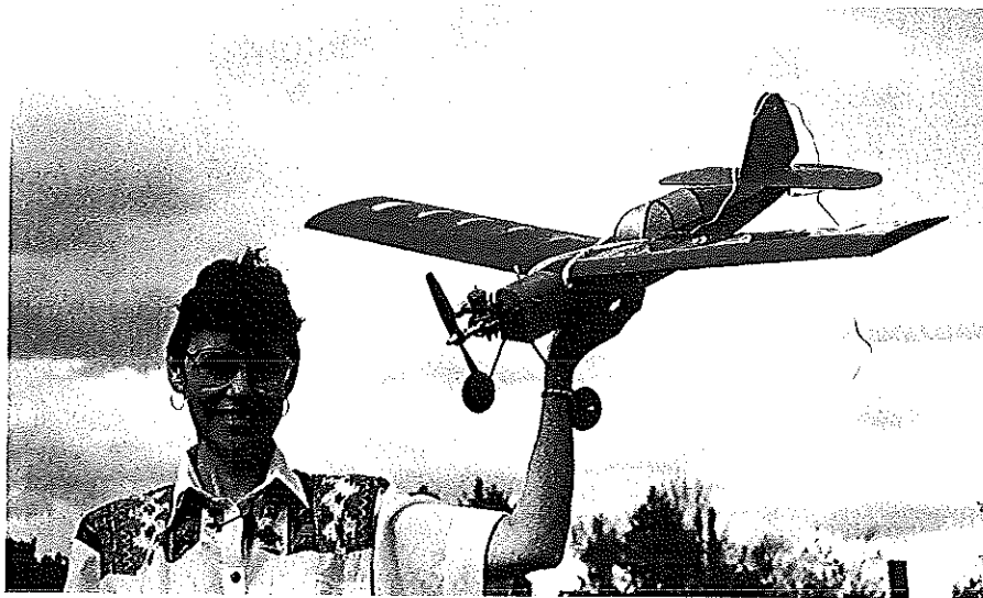
Author's wife Carol shows the RC Goat. Original CL model was published in November 1947 Air Trails . Several .049-.074 engines have been used.
