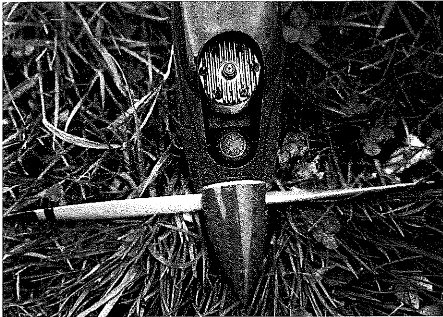
Note the neatness of the two-inch-diameter spinner, cowling ring, and engine air-intake hole. The prop is a Bolly 11 \frac{3}{4} x 3.8.
