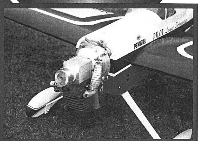
Sachs 3.2 on vibration isolation mounts. Two exhaust stacks exit from bottom. A special exhaust baffle is available.
