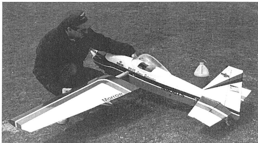
Lance begins field assembly by sliding aluminum-tube joiner through the fuselage. Lack of a cutout for the wing results in a stronger fuselage.
