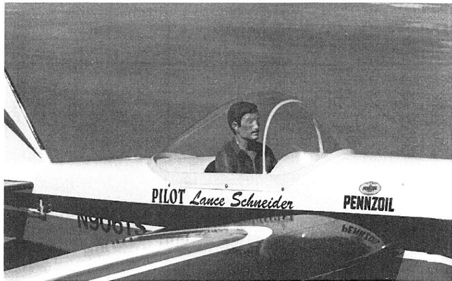
Pilot figure adds a touch of realism. The close-to-scale color scheme was accomplished with Coverite's 21st Century fabric and paint.
