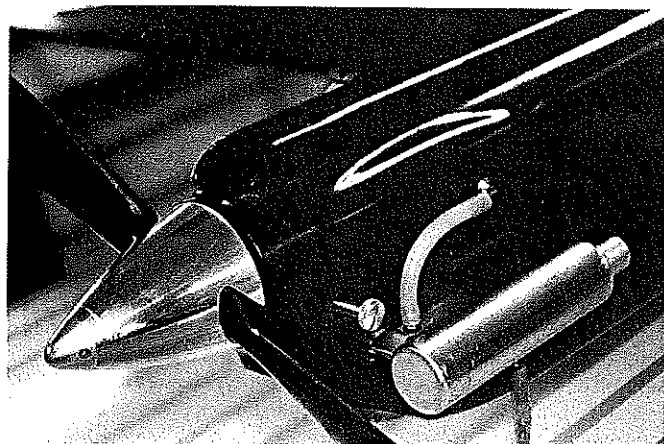
Power is a Big Jim Greenaway ST .60 with Big Art Adamisin muffler. Note valve cover blisters, similar to full-scale.
