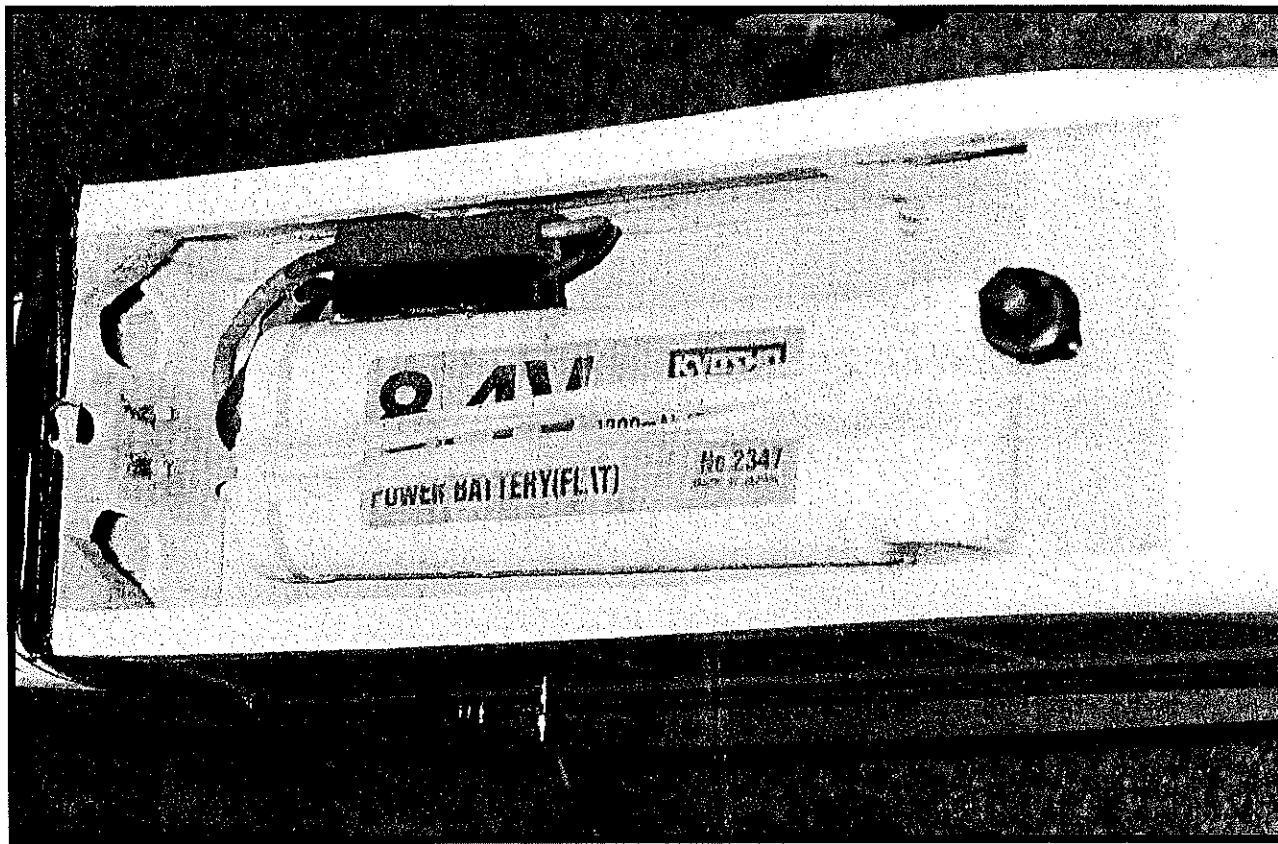
J-hooks and rubber bands anchor the battery to the tray, which in turn is screwed to the tray rails.
