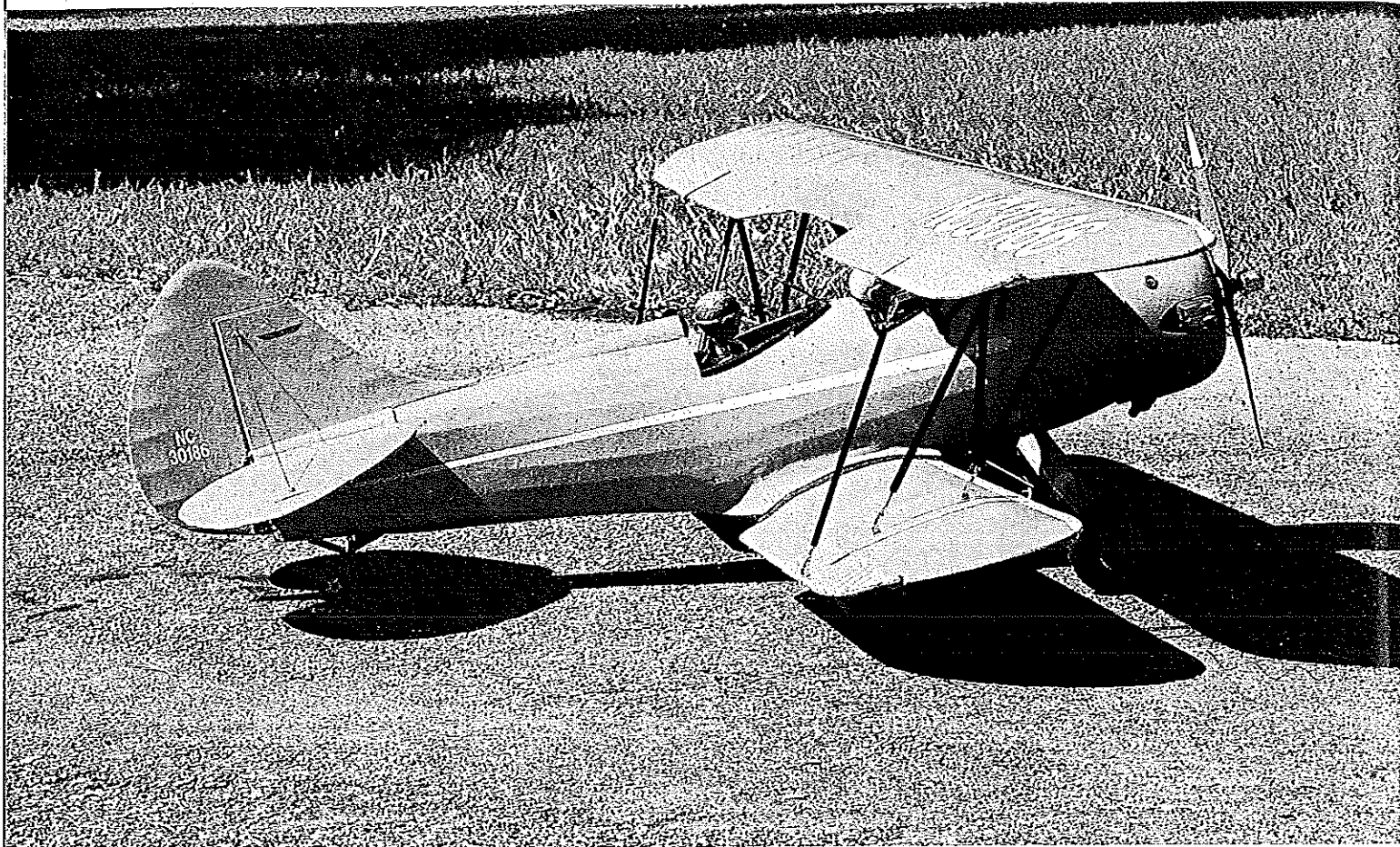
Paul Matt drawings were used as the basis for this 1:6.4 version. Clark Y airfoil was thickened to 15%.
