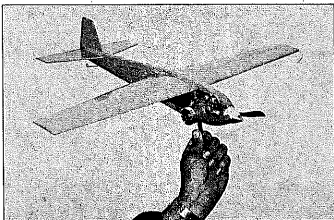
K&B .21 starts easily on crankcase pressure, runs steadily, and does well over 100 mph on an APC 7 x 6 prop.
