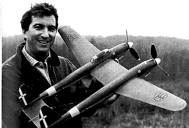
The S.M.92 regularly flies 50-65 seconds on two 27-inch loops of \frac{1}{8} FAI rubber. Model weighs 68 grams less rubber.
