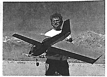
Bill Thompson (Modesto, California) powers his Senior with an O.S. .90. Design can handle a wide engine range.
