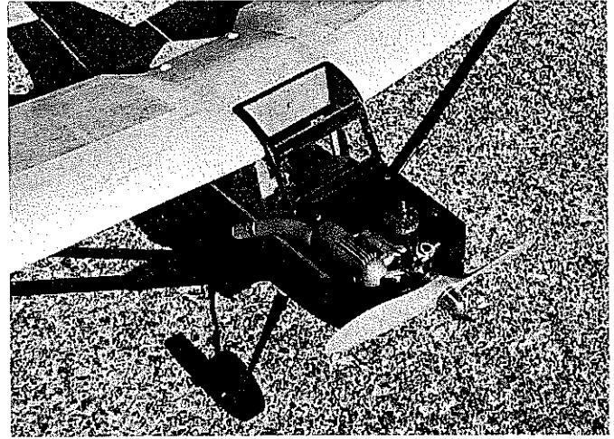
The O.S. .15 engine is perfect for the JN-1. Extension tube keeps exhaust oil off the airplane. Flying prop is a nylon 10 x 3. A small amount of downthrust was added after test flights.
