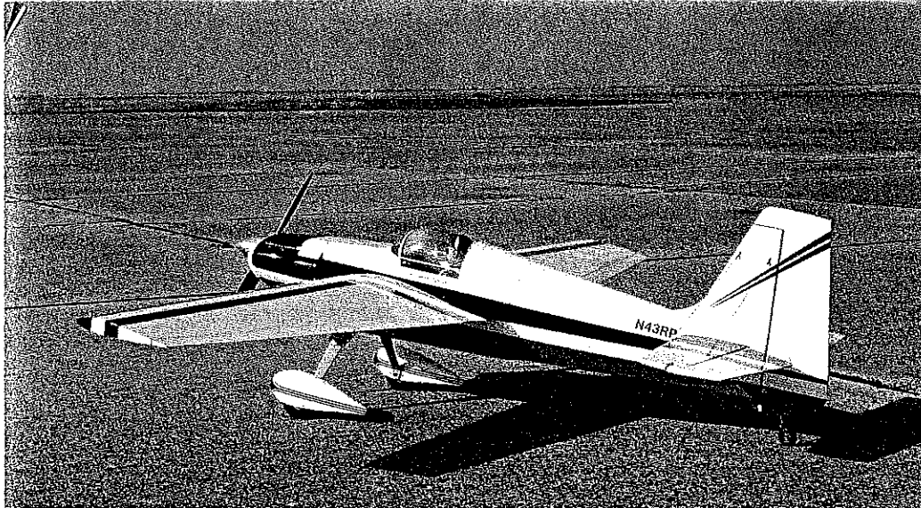
Three-quarters rear view of the model. Differences between this variant and the original Stephens Akro include a raised turtledeck and slightly enlarged tail surfaces.
