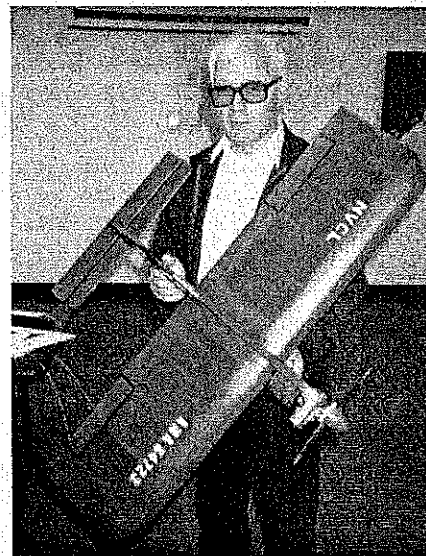
Al Jones also covered his model with silkspan. The first day's flying—Proto Speed and Endurance—did a good job of breaking in Jones's brand-new Fox .36 engine.
