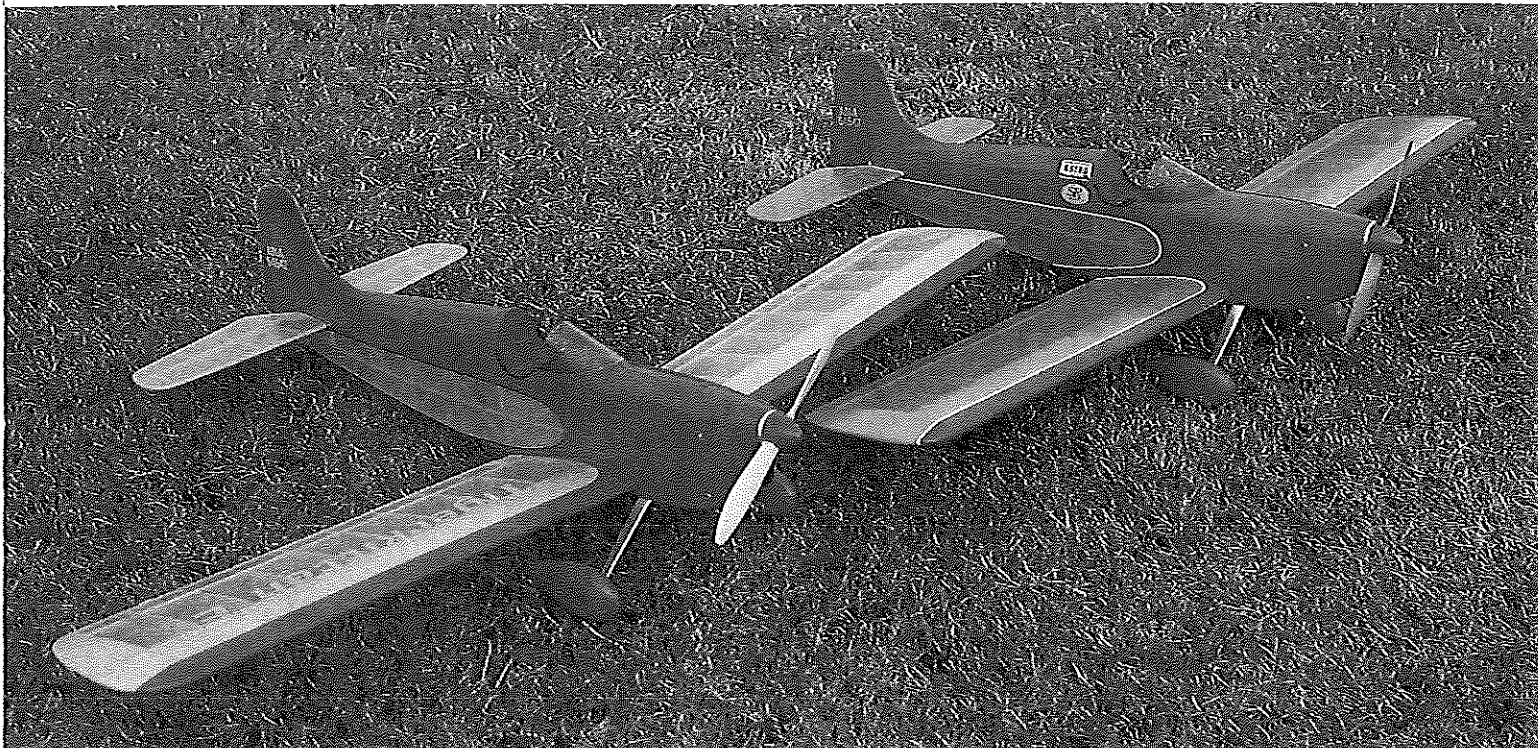
The two Tigerkitten "E" prototypes after an active flying session. The red-and-yellow model is covered with Sig Silray cloth dyed with Rit fabric dye and attached and sealed with clear nitrate dope. The color finish is Silts Polytone, a full-scale aircraft paint. The later version uses dope-finished orange Litespan and Bahama Blue Silts Polytone. With no fuel spills to worry about, the planes look great without any cleanup.
