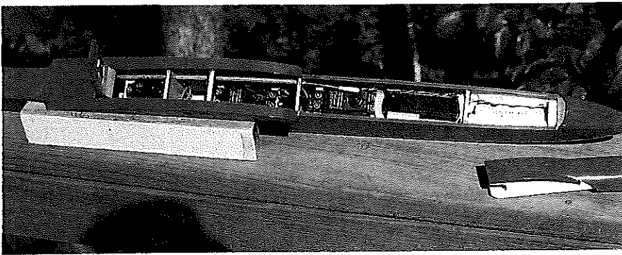
Looking down on the control layout. Shown are the 600-mAh ½AE battery, receiver, elevator servo, bulkhead-mounted switch, rudder servo, wing retainer hooks, and spoiler servo with pull strings over the ball links. Also note the small hook that holds down the rear hatch cover.
