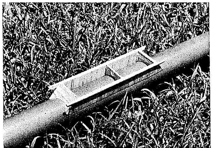
Left: Looking at the underside of the wing mount, you can see one of the two lengths of 1/8 x 1/16-in. balsa used to key the wing to the pylon mount. One piece is glued to each side of the wing. These pieces also serve to fill the gap between the top of the pylon and the bottom of the undercambered wing. Right: Construction details of the wing mounting pylon. The side rails are 1/8 x 3/16 spruce. An easy way to shape the base of the pylon is to wrap sandpaper around the motor tube and then sand the pylon base to a perfect fit before final installation.
