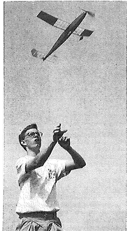
The author hand launching Embryo-omatic during a sequence of low-power test flights to adjust trim. It's important to have a bright, contrasting color scheme, as the airplane gets very small as it reaches its max altitude.
