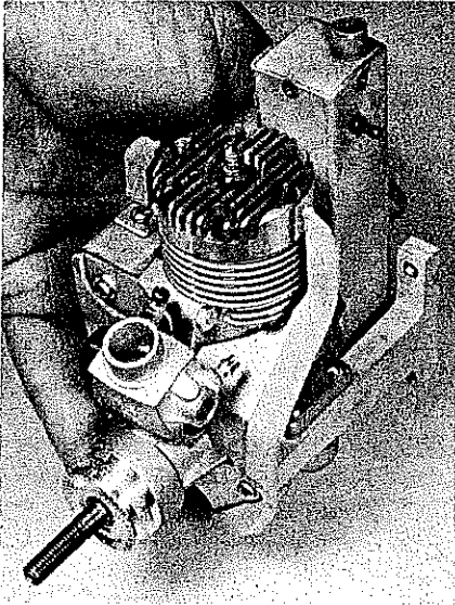
An O.S. .40 engine installed on Sig metal mounts. John Hunton's custom muffler nestles behind the side exhaust engine. The baffles increase air flow over the cooling fins.
