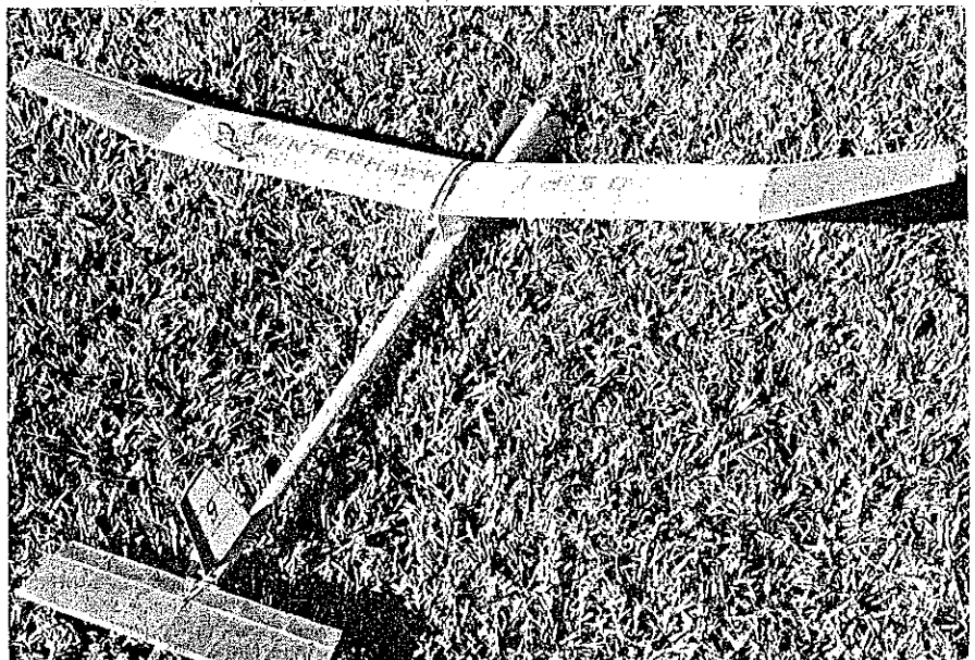
The Winter Hawk's wing uses a turbulated Sokolov airfoil. Wing area is 164 sq. in., and the aspect ratio is 13:1. A small gurney flap is used on the left tip panel to maintain a flat left glide.
