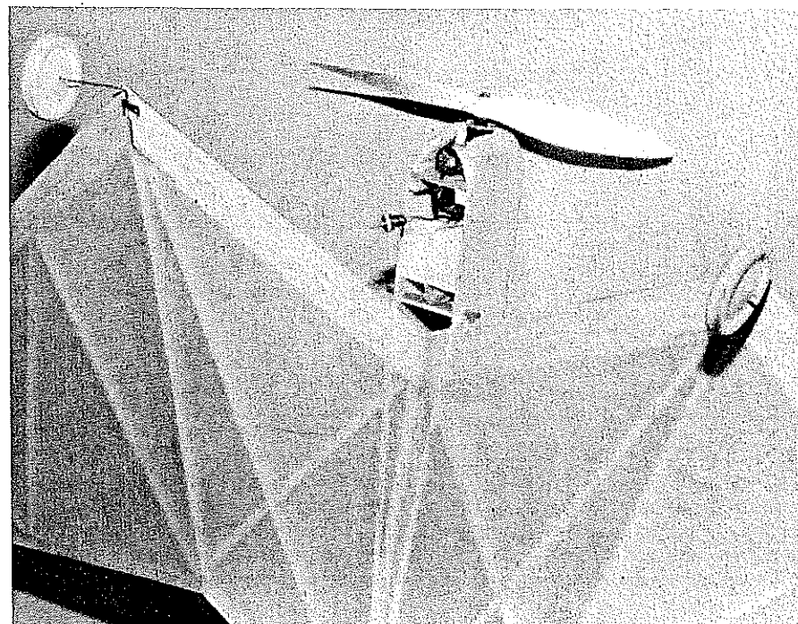
Close-up details of the underside of Noctule IIB showing the open bottom on the pod allowing air circulation around the CO 2 tank. Note the thread binding on the landing gear, the geometric wing structure visible through the tissue, and the rubberband wing mounting system.
