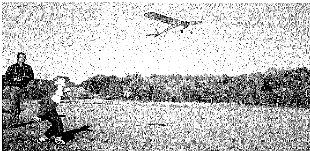
The author's son, Jeffrey, launching Lil' Ole Reliable. The airplane is extremely stable and will fly immediately upon launch. It can be hand launched or ROGed from a smooth surface.
