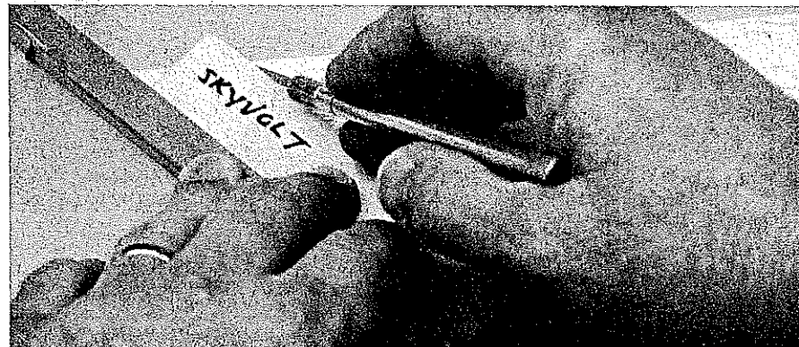
A template for accurately slicing the aileron sheeting at 45°. Butt the sheeting against the block, and let the template guide the knife. Top sheeting is wider than the bottom. See text.
